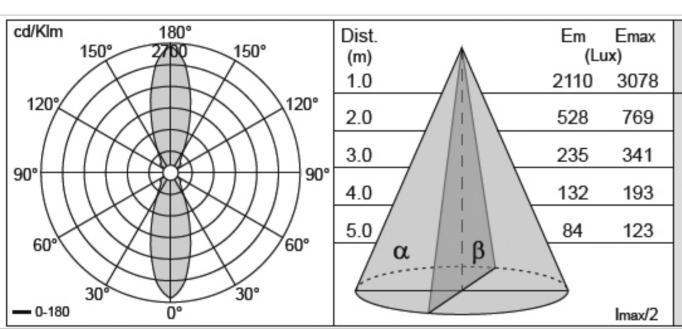
7450W/NC3.MB Flood CCT: 4000K Power: 50W System: 6400 Im Effic.: 128 Im/W Imax : 3078 cd/Klm LOR: 79 %  $\emptyset\alpha$ : 2.7m  $\emptyset\beta$ : 2.7m β: 29.9° α: 29.9°
